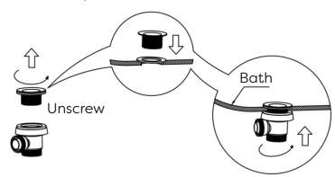
3. Place the overflow elbow (15) and rubber washer (16) on the bach of the bathtub. Screw in the overflow plug (17) into the overflow elbow (15). Push on overflow cover (18).
