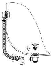
6. Fill the bath with water and check all joints to ensure there are no leaks. This is the best done in stages starting with a small amount of water before fully filling the bath
