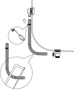
5. Tighten plastic nut (12) onto the waste body (9) and replace cover (from Step 1)
