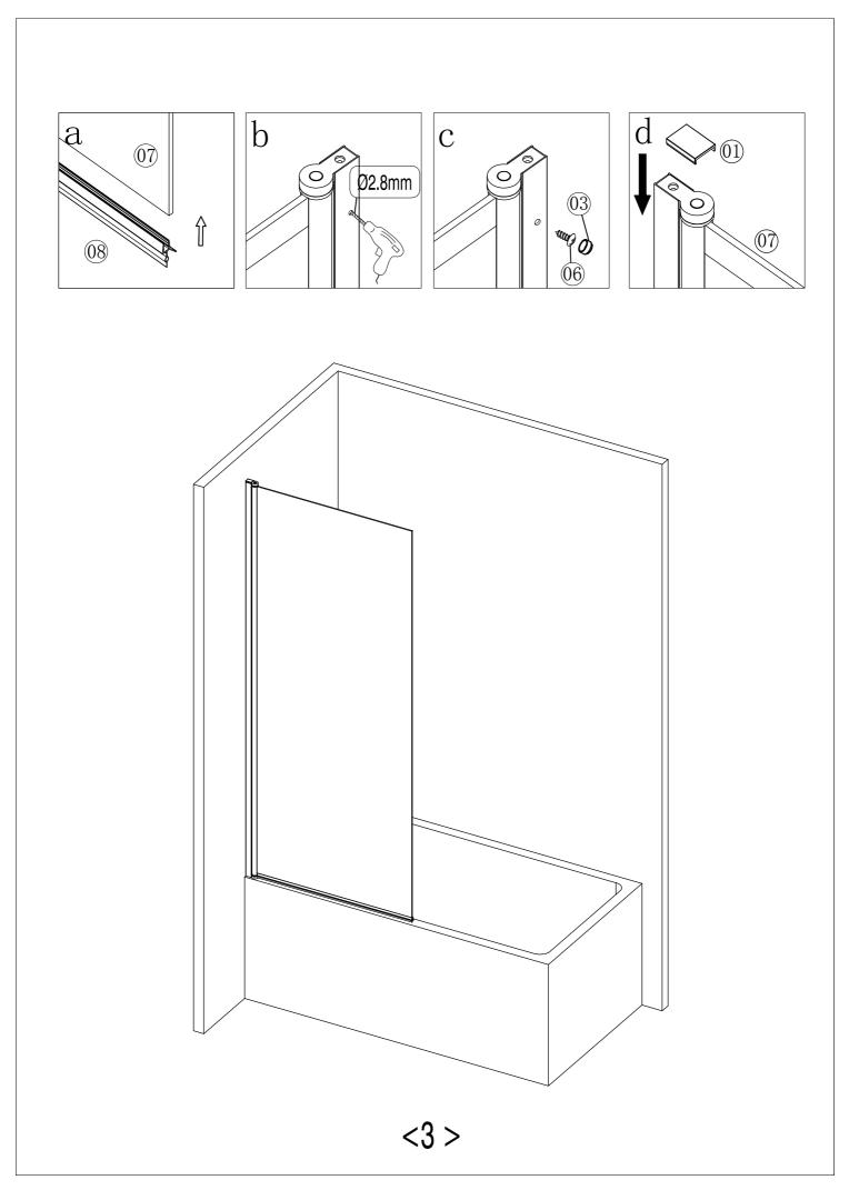
EXTERNALLY SILICONE SEAL THE WALL PROFILE WHERE IT MEETS THE WALL AND ALONG THE BOTTOM OF THE BLACK PROFILE. ALL IN A CONTINUOUS BEAD. DO NOT SILICONE INSIDE THE BATH SCREEN
