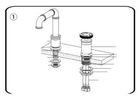
1. connect the hoses to the on/off valve, install the base ring and O ring, then lock the back nut
