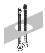
Feeding them through from underneath the sink hole, fit the water inlet flexi tail(s)/connector(s) by hand to the tap body.
