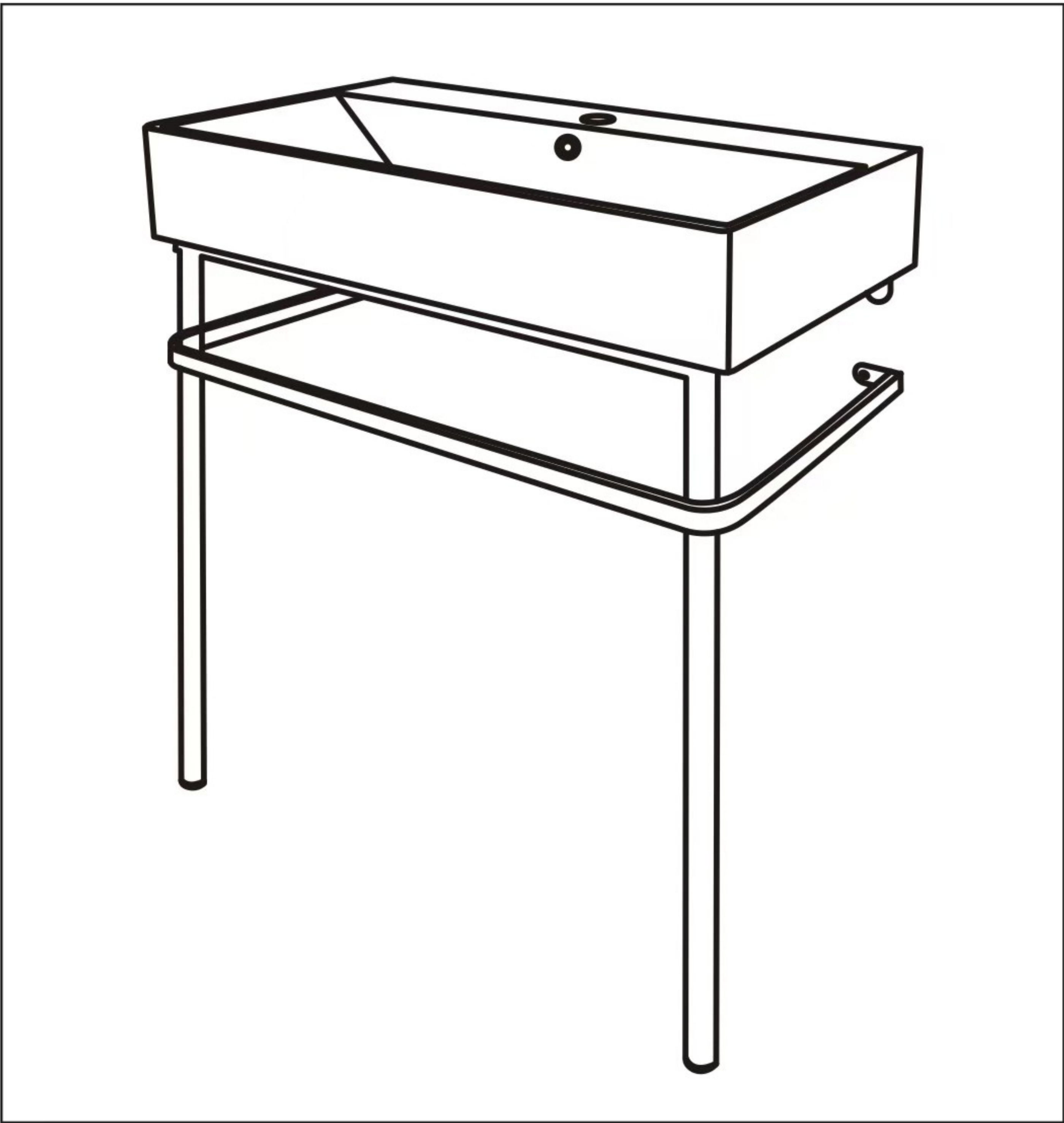
6.Put the ceramic washbasin on the support.
