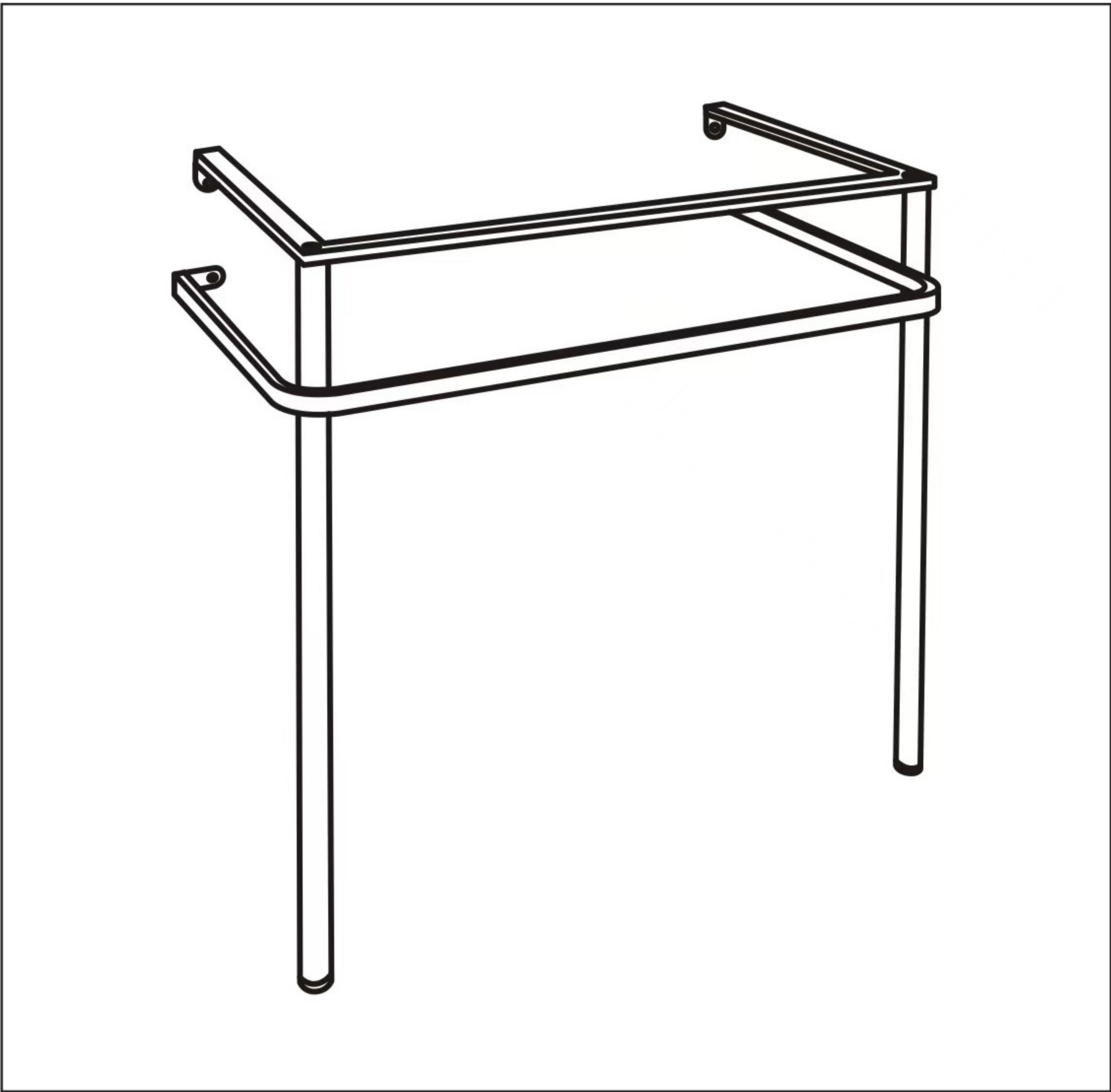
5.Attach the support to the wall with expansion screws.
