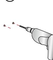
Using a 6mm drill bit, drill holes in the marked positions.
