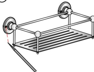
Determine the final installation position, mark the fixing hole positions in pencil.
