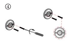
Screw in the stainless steel screws to secure the base to the wall. Please ensure that the screw heads are horizontally level.
