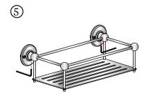
Insert the basket body into the base. Fix it with the allen key supplied.
