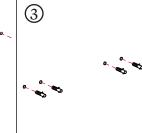
Insert the rawl plugs into the drilled holes.
