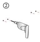
Using a 6mm drill bit, drill holes in the marked positions.
