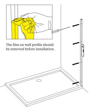
Place wall channel in position on the tray (10 - 15mm in from the outer edge of the tray), use a spirit level to ensure that they are vertical and mark all 4 fixing holes onto the wall.
