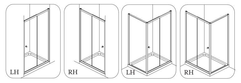
The Slider shower enclosure is reversible for left or right hand fitting. While the installation of the enclosure is LH, You just ignore the diagram below. For the RH installation, the diagram below should be followed.
