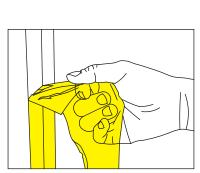
Remove protecting film Yellow protective plastic film on profiles are used to protect the plating finish to avoid scratching during installation. Please remove them before sealing.
