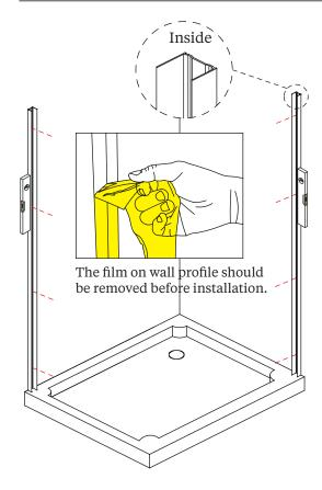
Remove both wall channels from the glass panel frame. <u>Note:</u> Ensure the longer leg of each wall channel is on the inside of the enclosure when fixing. Place each wall channel in position on the tray (10 - 15mm in from the outer edge of the tray), use a spirit level to ensure that they are vertical and mark all 8 fixing holes onto the wall.
