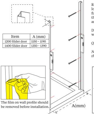
Remove both wall channels from the glass panel frame. <u>Note:</u> Ensure the longer leg of each wall channel is on the inside of the enclosure when fixing. Place each wall channel in position on the tray (10 - 15mm in from the outer edge of the tray), use a spirit level to ensure that they are vertical and mark all 8 fixing holes onto the wall.
