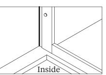
Sealing inside: Run a line of silicone sealant from top to bottom down the joint between the wall channels and tiles. Do not seal the enclosure to the tray on the inside.
