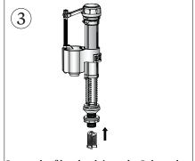
Insert the filter back into the Inlet valve.
