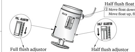
②Move adjustor down, flush volume increases. Move float up, flush volume decreases.
