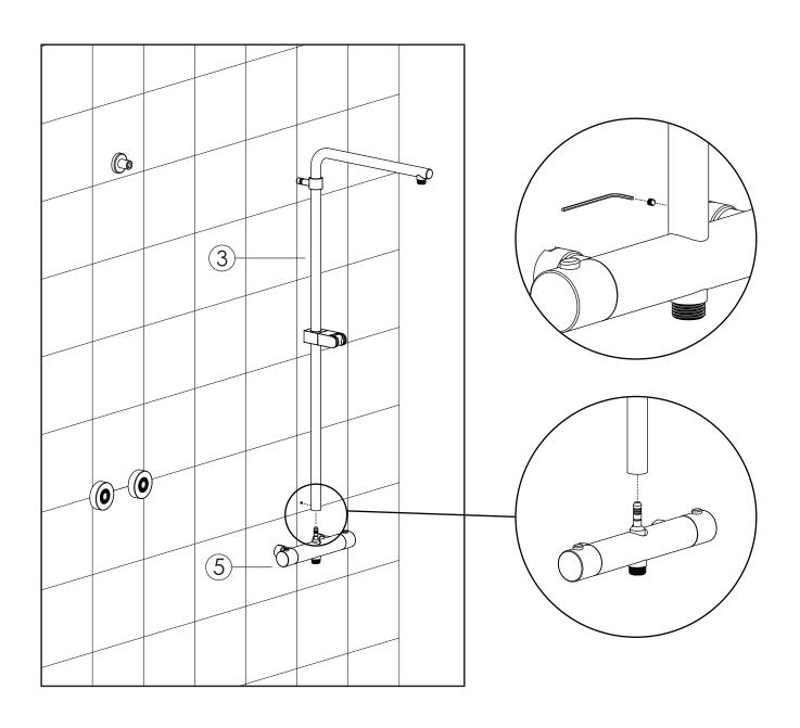
**STEP 4**Install faucet and Shower system tube to Wall connections.
