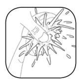
1. To break away scale deposite on a daily basis simply rub your thumb over the surface whilst the shower is running.
