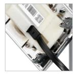
Locate the fixing lugs on the top of the controller into position at the top of the back plate and push the bottom of the controller into place. Hold the controller in position and secure to the back plate using the fixing screws at the base of the controller.
