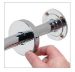
Ensuring the rubber washer is in the correct position, attach the shower head to the fixed arm and carefully secure using a suitable spanner, or a tool with smooth jaws, sufficiently to lock the head into position.
