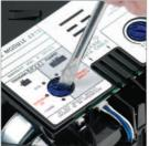
HP/Combi Digital processors fitted to balanced high pressure systems may be set to 'NORMAL HP', or for water economy, 'ECO' modes.
