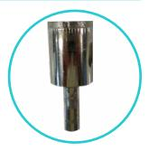
Position the hole saw on the tile at your chosen location and scribe around its edge.
