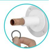
The O-ring must be positioned on the 15mm pipe flush to the fixing bush, not onto the fixing bush shaft.
