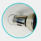
With the hole saw now straight, break the surface of the tile. If required, wet the tile and continue cutting. Repeat the process if necessary ensuring that the cutting area is always wet.
