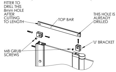
REMOVE THE FRONT SCREW FROM THE SCREEN TOP CAP AND THEN REFIT THROUGH THE 'U' BRACKET
