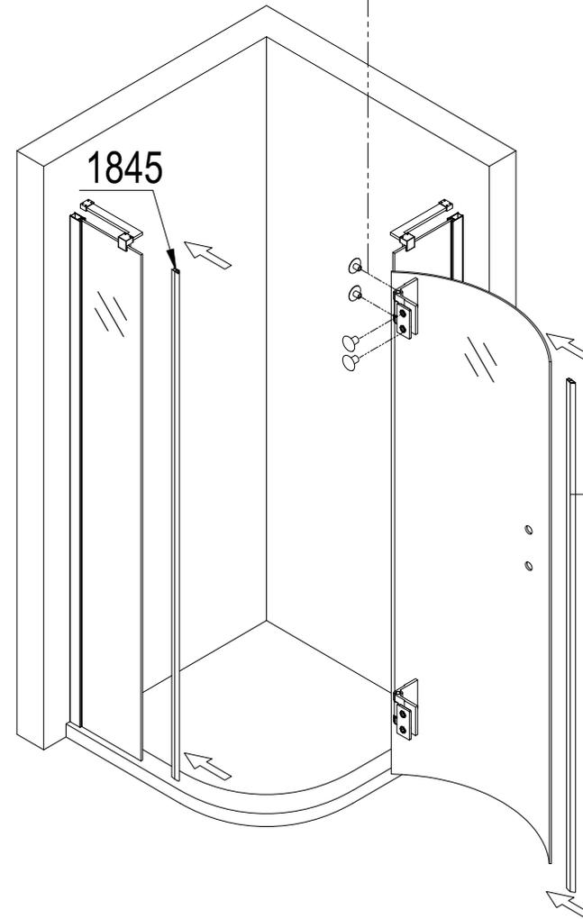
IT IS VERY IMPORTANT TO HAVE THE BOTTOM OF THE GLASS PARALLEL TO THE TRAY TOP FACE, IT MUST HAVE A 22MM EVEN GAP ALL THE WAY ALONG.
