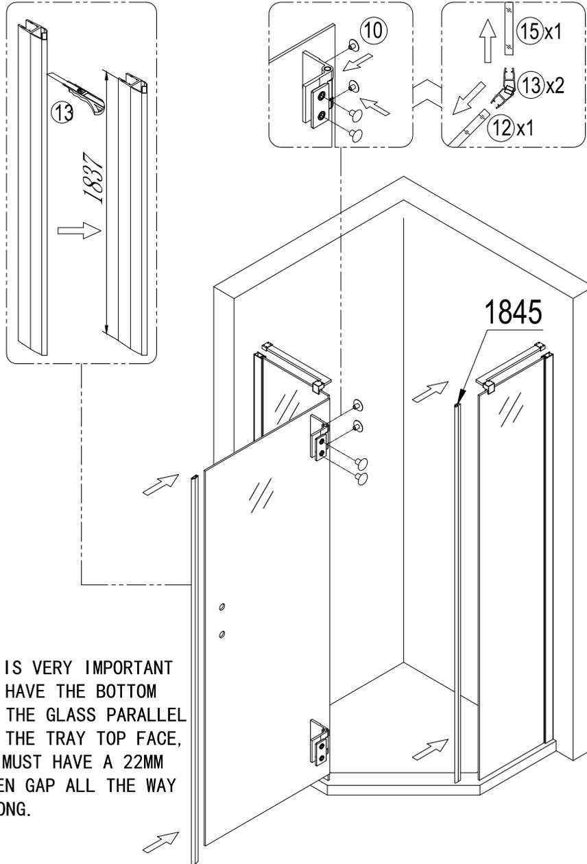
IT IS VERY IMPORTANT TO HAVE THE BOTTOM OF THE GLASS PARALLEL TO THE TRAY TOP FACE, IT MUST HAVE A 22MM EVEN GAP ALL THE WAY ALONG.
