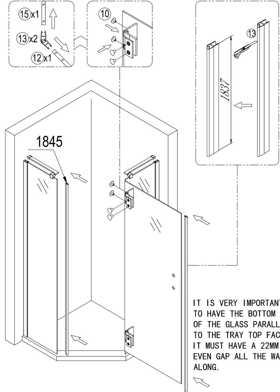
IT IS VERY IMPORTANT TO HAVE THE BOTTOM OF THE GLASS PARALLEL TO THE TRAY TOP FACE, IT MUST HAVE A 22MM EVEN GAP ALL THE WAY ALONG.
