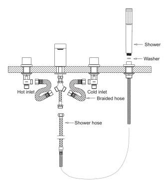
Connect the tee connector and the hot/cold control valves using braided hoses. Connect one end of the shower hose to the flexible tail of spout assembly and the other end to the shower, ensuring a washer is in.
