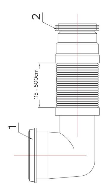
1. Flexible 90 Degree Pan Connector 2. Seal Ring
