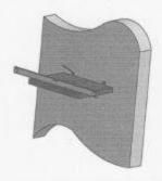
PLACE THE SHELF WITH THE BRACKETS IN THE SLOTS OF THE SHELF IN THE DESIRED POSITION ON THE WALL, USING A SPIRIT LEVEL TO ENSURE THE SHELF IS PLUMB, MARK THE POSITION OF THE BRACKETS AND FIXING HOLES ON THE WALL.
