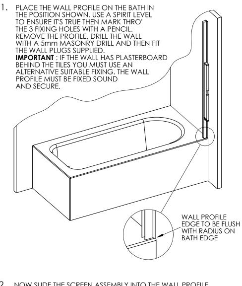
2. NOW SLIDE THE SCREEN ASSEMBLY INTO THE WALL PROFILE. THE BOTTOM EDGE OF THE GLASS PANEL **MUST** BE PARALLEL TO THE BATH TOP FACE. YOU CAN MAKE A WOODEN SPACER (18mm) TO FIT UNDER THE GLASS SO THERE IS AN EQUAL GAP ALL THE WAY LONG. THE SPACER WILL ALSO SUPPORT THE SCREEN PARALLEL WHILST YOU FIX IT IN PLACE.
