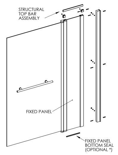
FIT THIS SCREEN IN EXACTLY THE SAME WAY AS STEPS 1,2 &3 BUT FIT THE FIXED PANEL BOTTOM SEAL IN PLACE BEFORE YOU SLIDE IT INTO THE WALL PROFILE (\* THIS SEAL IS OPTIONAL AS YOU CAN USE SILICONE SEALANT INSTEAD).
