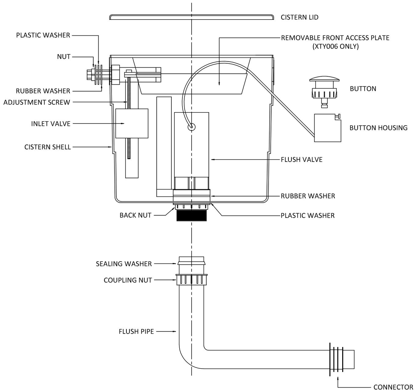
**ASSEMBLE THE CISTERN AS ABOVE AND MARK THE POSITION OF WHERE THE CISTERN IS TO BE FITTED. USE THE BRACKET AND FIXING HOLES TO FIX THE CISTERN INTO THE W.C UNIT OR WALL CAVITY.**
