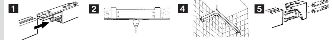
1. Lightly assemble the chosen rail arrangement, including ceiling support socket and wall brackets. To join rails, push the cruciform dowel into the center of one rail, then loosen screws of joining piece and slide into top channel.
