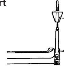
1. Locate the nearest suitable joist above the rail for the ceiling bracket and mark the ceiling. Use a 3mm drill to make a pilot hole and screw bracket to the ceiling. In some cases it may be necessary to fit a cross bearer between the joists for the ceiling bracket.
