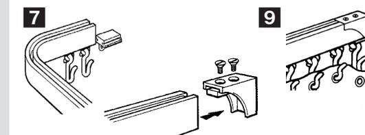
6. Align second rail with the dowel and joining piece and push the two rails together.
