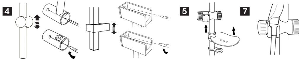
4. Fit the rail into the lower bracket. Place the remaining bracket on top of the rail making sure it is located into the bracket slot. Ensure the hole position is vertically aligned and mark the wall. Remove the rail then drill and plug the wall.
