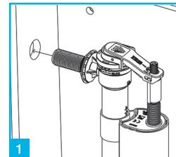
Remove the plastic washer and nut from the thread and place the valve in the correct position inside the cistern ensuring the conical rubber seal sits evenly inside the hole.
