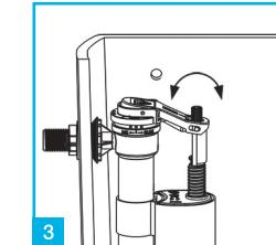
The water level can be adjusted by turning the adjustment screw (clockwise for more water, anticlockwise for less water).
