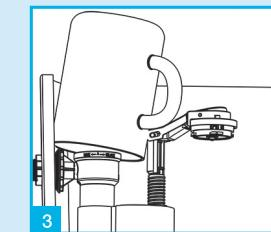
Turn water supply on and off to clear any debris. Hold a cup over top to prevent any splashing.
