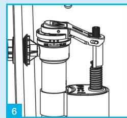
Refit top assembly complete with diaphragm.
