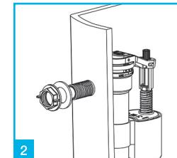
Secure the valve to cistern by replacing the plastic washer and screwing the nut to the thread. Do not over tighten.
