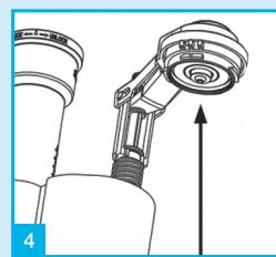
Remove diaphragm washer and clean with water or replace.
