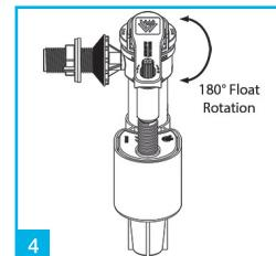
The valve has a float rotation system, allowing the float to be rotated 180°. This is really beneficial if space is an issue.
