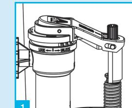
Turn off water supply and set access wheel to unlock.
