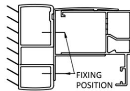
WHEN CORRECTLY ALIGNED, MARK THROUGH THE FIXING HOLES SHOWN ABOVE ON TO THE EXTENSION PROFILE.
