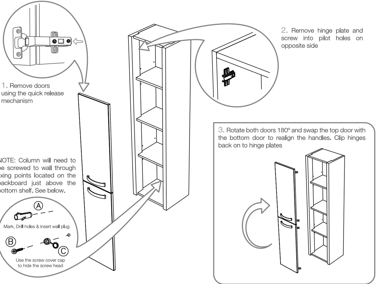
1. Remove doors using the quick release mechanism
