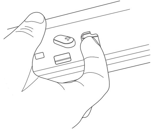
6 Gently slide the drawer outwards and upwards to remove fully from runner.
