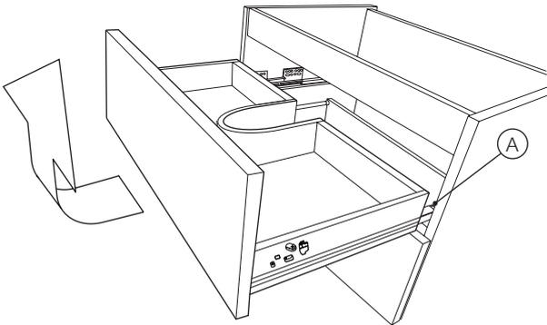
7 Unscrew the CAM screw on the underside of the drawer
