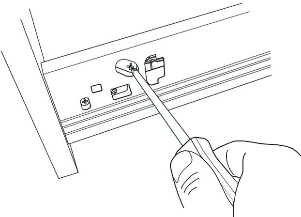
9 Release the adjustment rail (diagram 10) then pull the fascia away from the body of the drawer.
