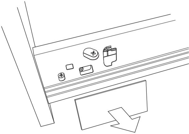
5 Squeeze the lever on each side of the drawer to release from runner
