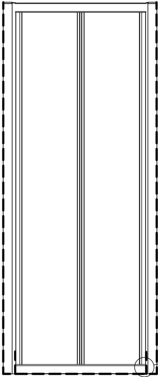
EXTERNALLY SILICONE SEAL THE WALL PROFILES WHERE THEY MEET THE WALL AND THE BOTTOM PROFILE WHERE IT MEETS THE TRAY. ALL IN A CONTINUOUS BEAD.
