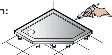
\* If the 'easyseal' water sealing strip is not installed, please seal joints between tray and wall with an anti fungal silicone sealant and allow to set.
