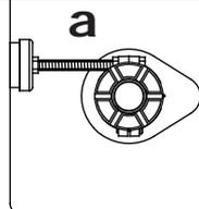
**a:** Ensure the panel fixing rod is located at 90° to the edge of the tray as shown above.
