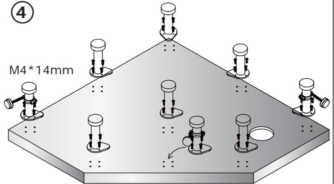
Screw the feet in position with the screws provided. Ensure that the feet that have panel fixing rod attached, are placed around the bended edge where the panel will meet.
