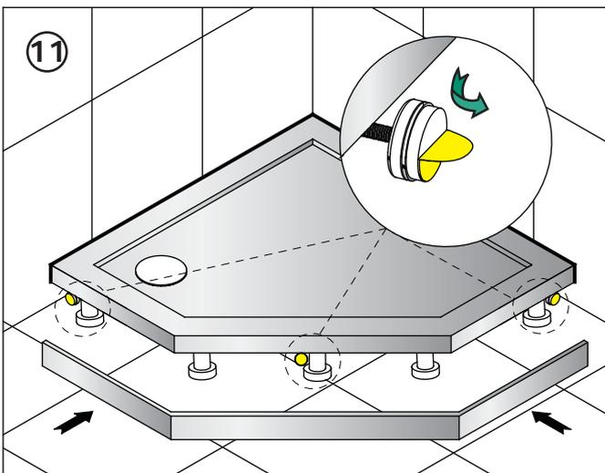
Remove the protective cover from the adhesive tape. Fix the panel pushing it firmly on to the adhesive pads.
