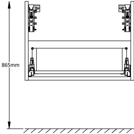
Fix Wall Hanging Plates as shown above. Check the type of wall you are fixing into and use suitable fixings (Not supplied).
