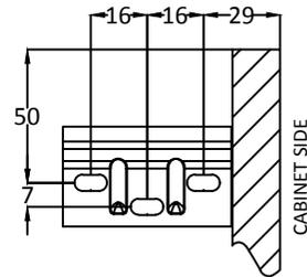
You may need to lengthen the hook's protrusion. To do so, turn screw 'B' anti-clockwise. Tighten screw 'B' to fit the cabinet to the wall. You may need to make some fine adjustments once the cabinet is fitted. Turn screw 'A' clockwise for DOWN and anti-clockwise for UP.
