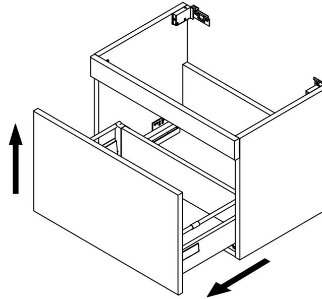
Remove drawer from cabinet prior to fitting unit to the wall. Pull-out the drawer to its full extension and gently lift the drawer box upwards until it disengages from the runner.
