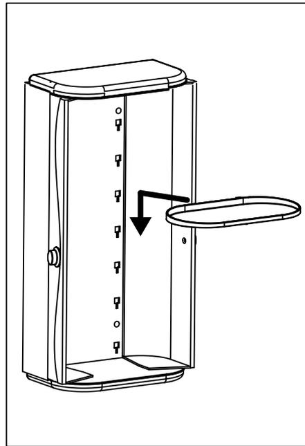
**Assemble the shelves into the cabinet to finish the installation.**
