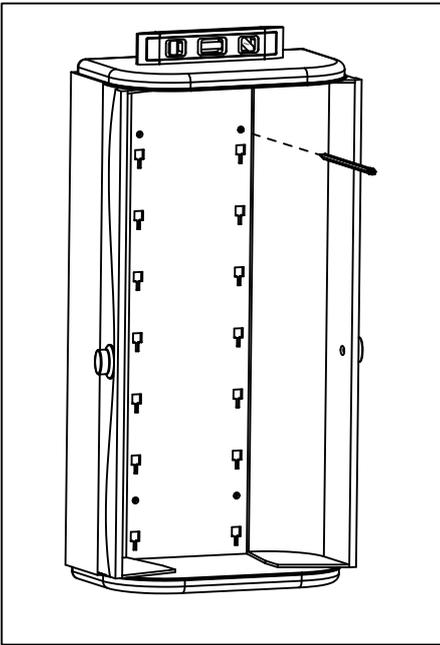
**Door opening - Grasp both door handles and rotate the doors carefully outwards. Place the cabinet in the desired location, level and mark screw hole positions.**
