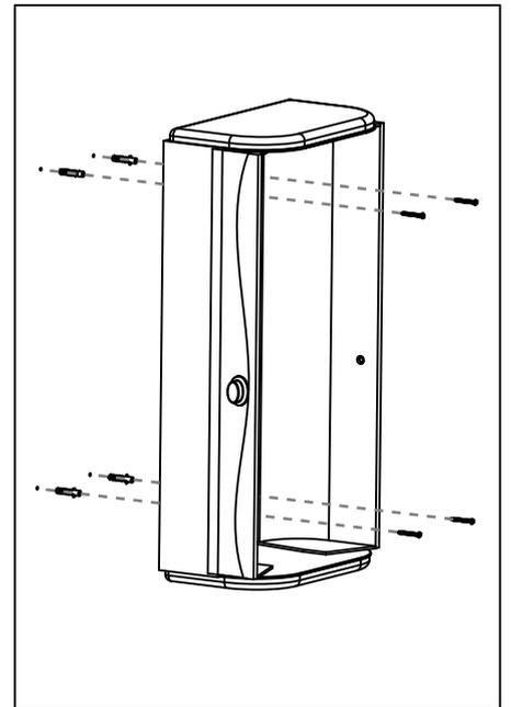
**Insert the wall plugs into the wall then screw the cabinet into position. Do not over-tighten the screws.**
