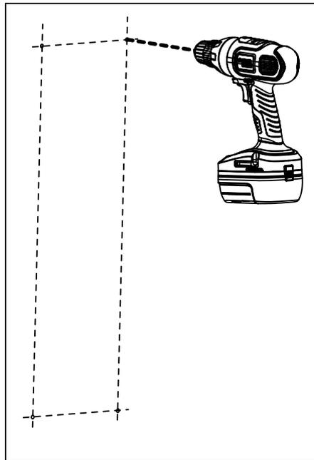
**Drill the holes using a 6mm drill bit to a suitable depth for the wall plugs.**
