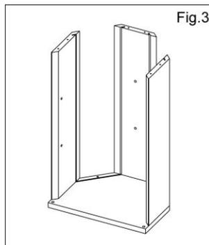
3. Secure side panel and back panel to the base using 4 fixing screws. (Screws mounted from underside of base. To improve strength place small amount of glue on underside of side panel before securing into position.)
