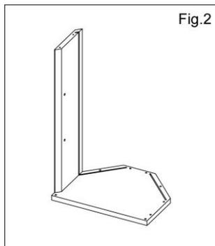
2. Secure side panel to base panel using two fixing screws. (Screws mounted from underside of base. To improve strength place small amount of glue on underside of side panel before securing into position.)
