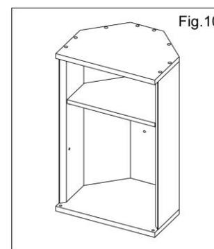
10. Insert shelf supports into hole recesses and ensure all supports are aligned accurately. Place the shelf in the cabinet and lower onto the shelf supports. (Door not shown.)
