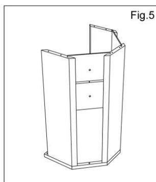
5. Slide the two strengthening batons into the channels at the rear of the cabinet with the pilot holes facing towards the top of the cabinet. Not to be secured into top panel at this stage.
