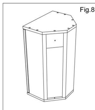
8. Slide the hanging batons up to the top panel and secure into position with the two remaining fixing screws.
