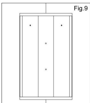
9. Hold the cabinet against the wall in its desired location and check that it is straight and level. Open the door(s) and mark the wall using the holes in the back of the cabinet as a guide. Drill 40mm deep holes in marked positions using a 6mm masonry drill and insert wall plugs. Align the holes in the back of the cabinet with the wall plugs. Insert the screws through the washers and holes in the back of the cabinet and screw in position.
