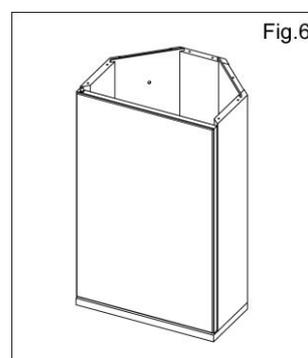
6. Place one of the door pivot pins into hole recess situated on the base panel. (The pivot pin bush needs to be located in the recess before inserting the pivot pin) Locate mirrored door onto pivot pin and place second pivot pin into the top of the door before securing the top panel.
