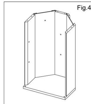
4. Locate the backing boards into the recesses on the side panels and back panel. Screw fixing holes to be positioned at the top of the cabinet. (Note- if positioned incorrectly the cabinet cannot be hung.)
