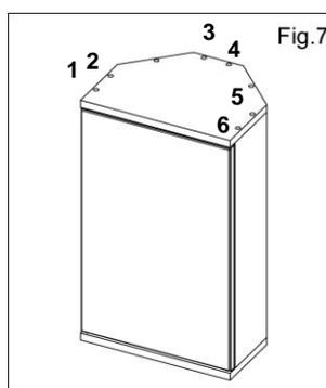
7. Place top panel onto cabinet carcass ensuring all screw holes, recesses and pivot pin bush are accurately aligned. Secure the top panel to the side panels and back panel. (Six fixing screws required.) To improve strength place small amount of glue on underside of side panel before securing into position.)
