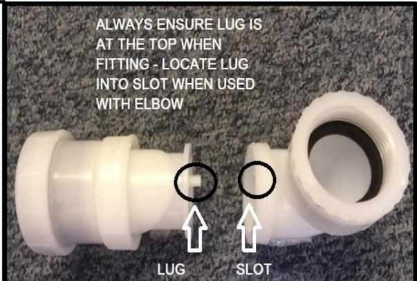
**INSTRUCTIONS - REMOVE ELBOW TO USE AS INLINE TRAP. REMOVE PLASTIC BUSH FROM ELBOW FOR 1 ½ THREADS. SELECT APPROPRIATE BLACK WASHER FOR RELEVANT SIZE OF WASTE PIPE. IMPORTANT: ALWAYS POSITION LUG AT THE TOP OF FITTING. DO NOT TOUCH INTERNAL RUBBER MEMBRANE WITH FINGERS OR OTHER OBJECTS.**
