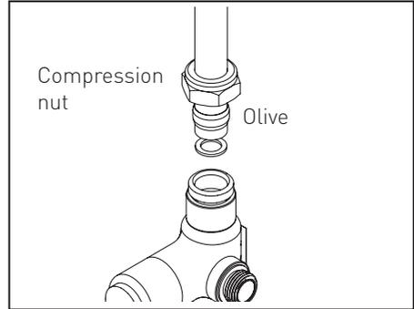
2. Tighten the nut fully using a suitable spanner to ensure a water tight seal.
