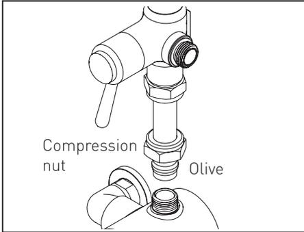
1. Push the short connecting tube into the top outlet on the shower valve (not supplied) ensuring the nut and olive are fitted to the connecting tube.
