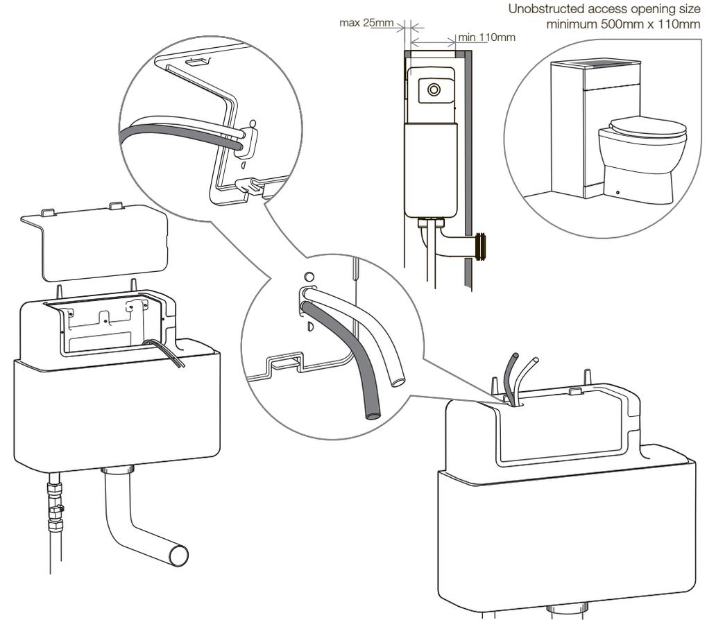
**installation of pneumatic push-button**
