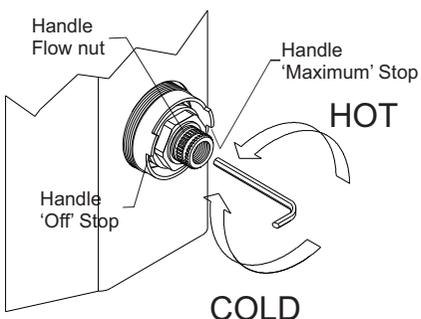
1. Use the handle to rotate the flow nut clockwise to turn off the thermostatic shower valve.
