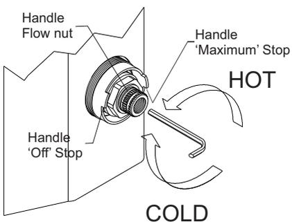
1. Use the handle to rotate the flow nut clockwise to turn off the thermostatic shower valve.
