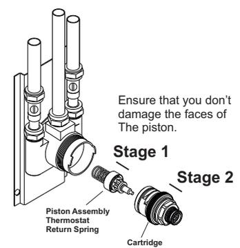
If your thermostatic mixing valve fails to operate it could be the result of incorrect installation. Please refer to installation and site requirements.
