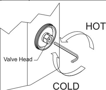
1. Whilst depressing the Time flow push button insert the allen key into the temperature adjusting screw in the front of the 'Valve Head' and adjust the outlet temperature to 41°C. Turn the adjusting screw allen key clockwise for a cooler temperature, anti-clockwise for warmer temperature.
