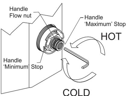
1. Use the handle to rotate the flow nut anti-clockwise until the thermostatic cartridge is fully open (The flow nut will no further rotate anti-clockwise).
