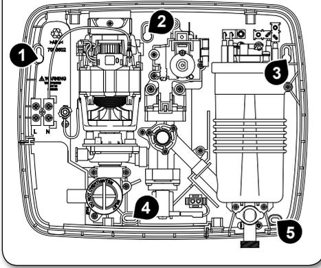
After choosing the site for the shower, use the backplate as a template (**fig.11**) and mark the four fixing holes 1, 3, 4 and 5.
