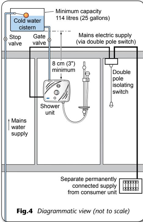
**Fig.4** Diagrammatic view (not to scale)
