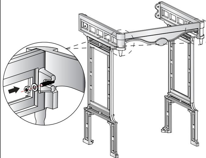
**2** Determine the final installation position. Ensure the basin stand is level, mark the fixing holes position onto the wall and floor in pencil.
