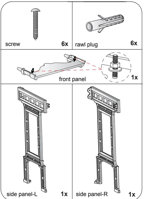
**1** Assemble the front panel and the side panels together as the diagram below. Tighten the nut with a spanner.
