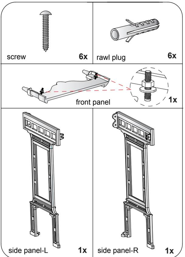
**1** Assemble the front panel and the side panels together as the diagram below. Tighten the nut with a spanner.
