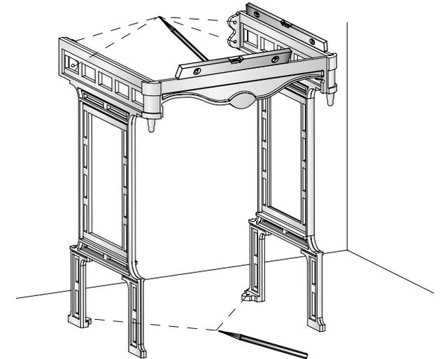
**3** Using a Ø8mm drill bit, drill holes on the marked positions. Insert the rawl plugs into the drilled holes.
