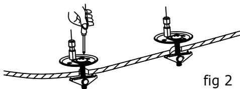
2. Using a crosshead screwdriver tighten the pan seat fixings. Make sure there is still slight movement in the pan seat fixing for final alignment as per figure-2.
