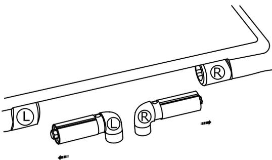
3. Insert the soft close barrel into the housing hole on each side of left and right.
