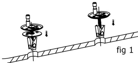
1. Insert the pan seat fixings into the pan seat fixing holes as per figure-1 by clenching the butterfly clips (C) together and pushing into pan seat fixing holes. The butterfly clips will open upon the other side of the pan.
