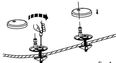
5. Using a crosshead screwdriver completely tighten the pan seat fixings taking care not to move their position. Fit the pan and seat fitting covers (B).
