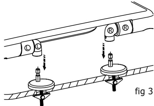
4. Slot soft close barrels on to location pins on pan seat fixings. Align seat and lid to the pan, and ensure that when seat and lid are open they lean back against the cistern and stay open. Carefully remove the toilet seat assembly.
