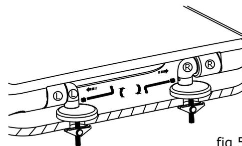
6. Place seat and lid back on to the location pins on the pan fixings and then use hex key provided to tighten grub screws found on the soft close barrels as per figure-5.
