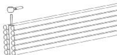
Using a hammer & steel rod to remove the centre block piece
