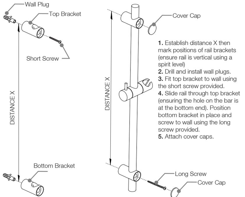
1. Establish distance X then mark positions of rail brackets (ensure rail is vertical using a spirit level)
