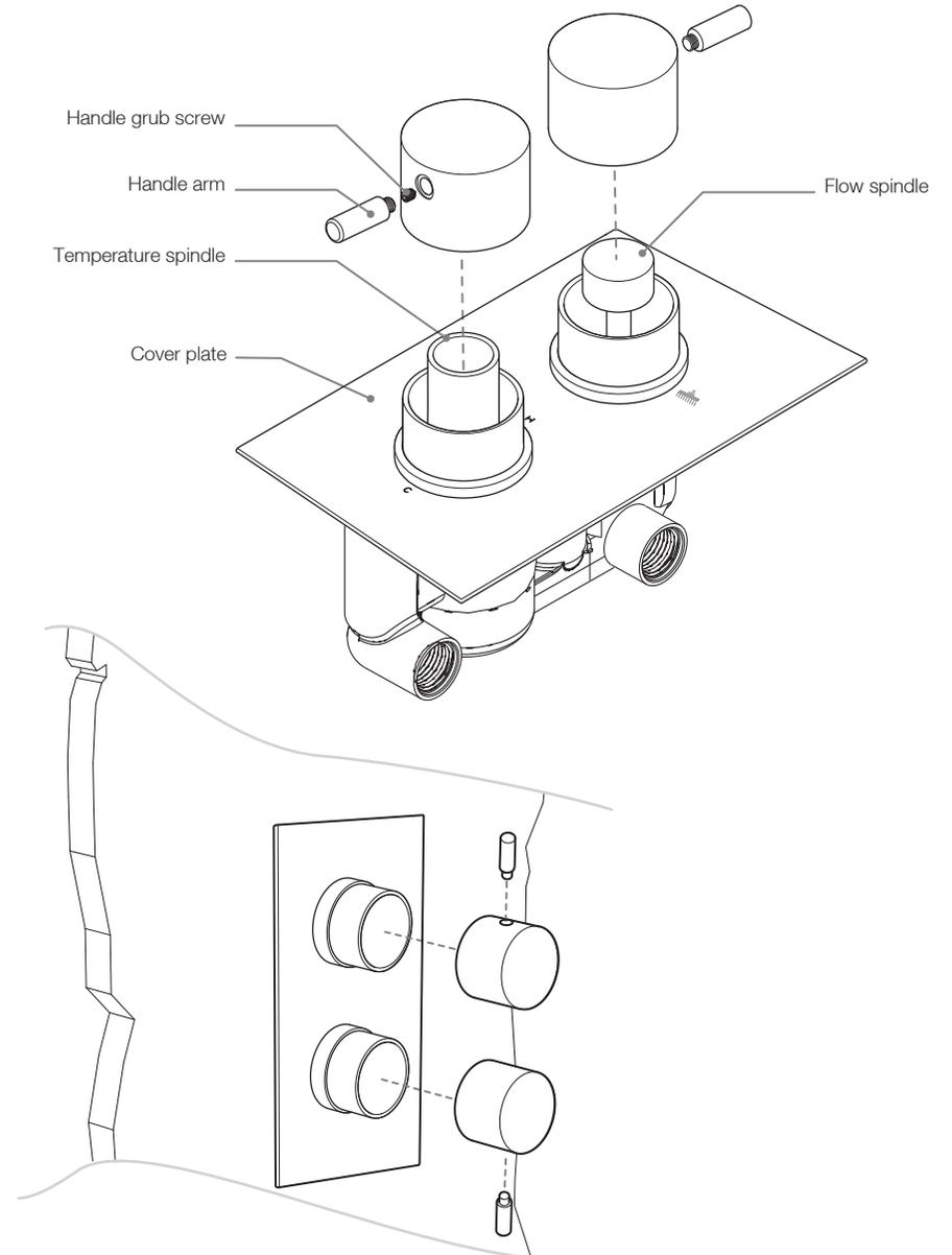
10. Apply a small bead of silicone behind the front cover plate and slide over the body into position. Smooth off against the wall finish.
