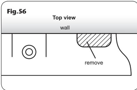
If a surface cable entry from the top is required then the relevant hole in the backplate will need to be cut out (**Fig.56**).
