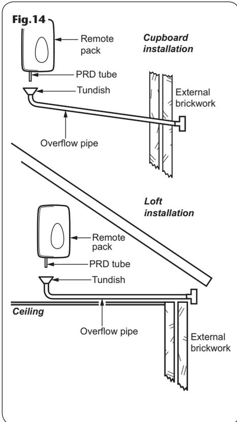
In the event of the PRD operating, turn off the electricity and water supplies to the shower at the isolating switch and stopvalve. Contact Customer Service for advice on replacing the PRD.
