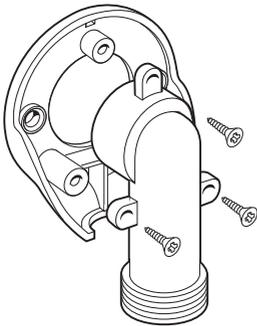
Screw the bulkhead assembly onto the threaded connector temporarily. Mark the position of the two fixing holes (**Fig.28**) securing the bulkhead to the wall.
