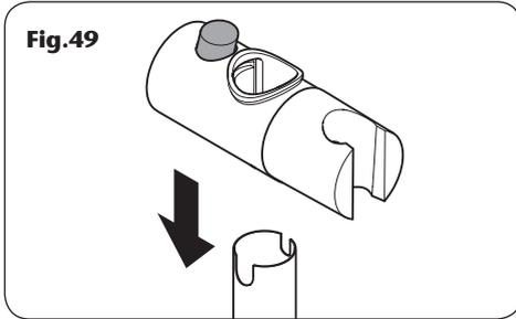
Slide the hose retainer onto the lower rail section. Fit the showerhead holder onto the riser rail section, press and hold the button on top of the holder to release the locking mechanism, then slide onto the rail (**Fig.49**). Release the button to lock the holder in place.
