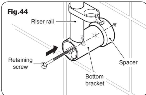
**INSTALLATION OPTION 3: THROUGH THE CEILING FITTING (LONG)****COMPONENTS**
