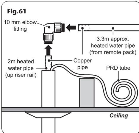
In the loft, trim the 2 metre heated water pipe excess to length. Insert the 8 mm copper pipes into the end of both water pipes and then push fit both ends into the 10 mm fitting (**Fig.61**).
