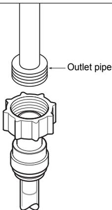
Fit the clear plastic PRD tube through the can outlet pipe boss situated at the rear of the outlet pipe (**Fig.24**) and push firmly on to the PRD outlet.
