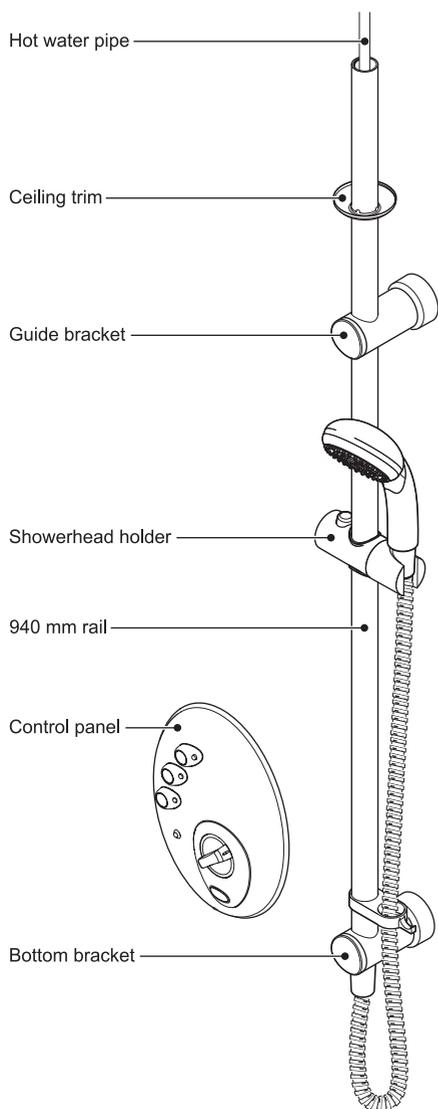
**Fig.10** Through the ceiling fitting (long)
