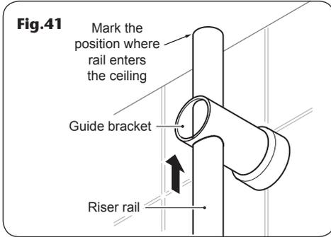
Slide the riser rail up through the guide bracket until it touches the ceiling (**Fig.41**). Using a spirit level, align the riser rail vertically and mark the centre hole position of the rail on the ceiling. Remove the rail.
