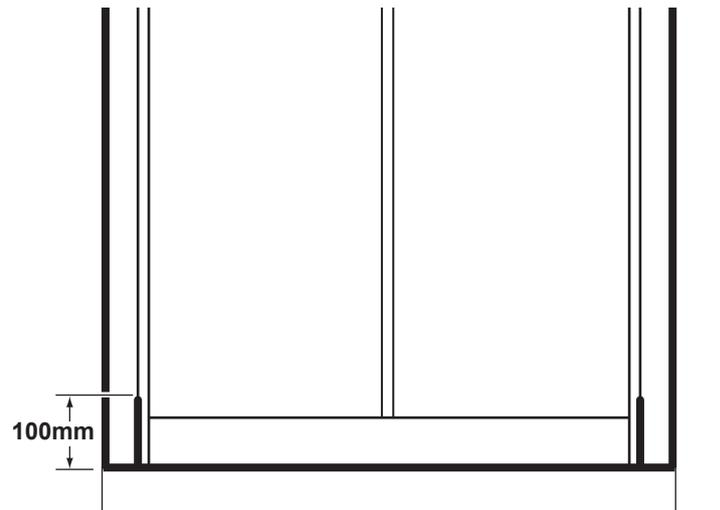
**Sealing outside:** Run a line of silicone sealant from top to bottom down the joint between the wall channels and tiles. Run a line of silicone sealant 100mm up the joint where the door slots into the wall channels. Run a line of sealant along the base in the joint between the bottom of the enclosure and the tray, from wall to wall.
