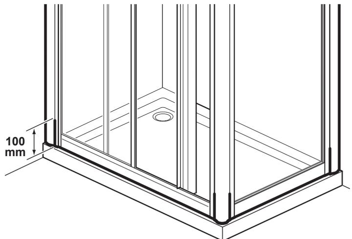
**Sealing outside:** Run a line of silicone sealant from top to bottom down the joint between the wall channels and tiles. Run a line of silicone sealant 100mm up the joint where the door and side panel slot into the wall channels and corner post. Run a line of sealant around the base in the joint between the bottom of the enclosure and the tray, from wall to wall.
