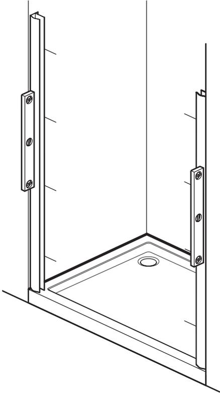
Remove both wall channels from the door frame. Place each wall channel in position on the tray (10 - 15mm in from the outer edge of the tray), use a spirit level to ensure they are vertical and mark all 8 fixing holes onto the walls (holes inside).
