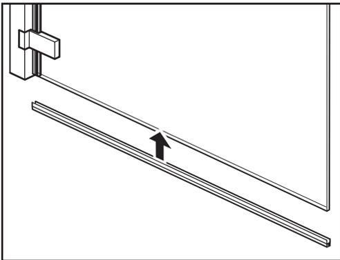
Remove the water seal (D) from the front edge of the glass and push fit onto the bottom of the bath screen. Ensure the seal is flush with the back edge of the glass. If necessary, trim the seal using scissors to get a good fit against the black seal.
