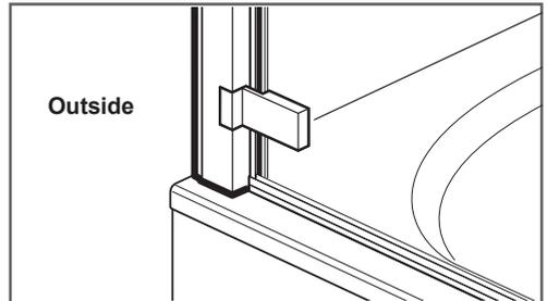
**Outside only:** Run a line of silicone sealant along the joint between the bottom edge of the wall channel and bath rim.
