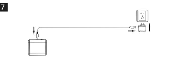
To recharge the battery remove the battery pack from the mounting bracket by gently pushing up and then pulling towards yourself. Then connect the USB cable to the charger and light. The indicator light will be red whilst charging. When finished charging the light will turn green. Charging time: 4hours, continuous working time: 7.5 hours.
