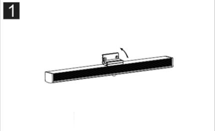
Turn the light so that the screw holes are accessible, as shown above. The light can be turned to a desired position after installation.
