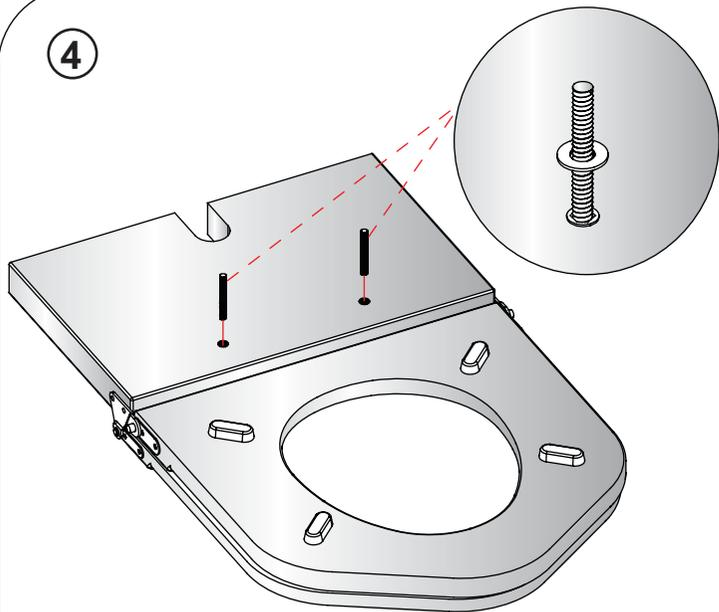
Screw the fixing bolts into the plugs, and attach on the washer.
