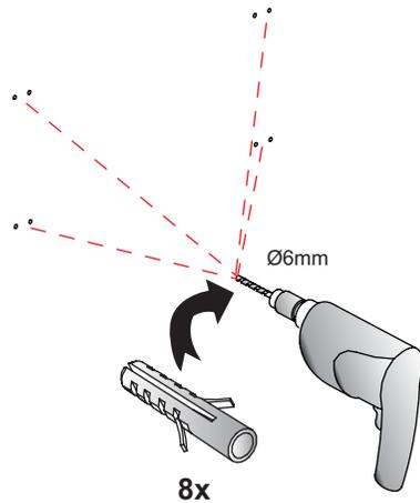
Drill holes using the Ø6mm drill bit following the marked positions, and insert the wall plugs.
