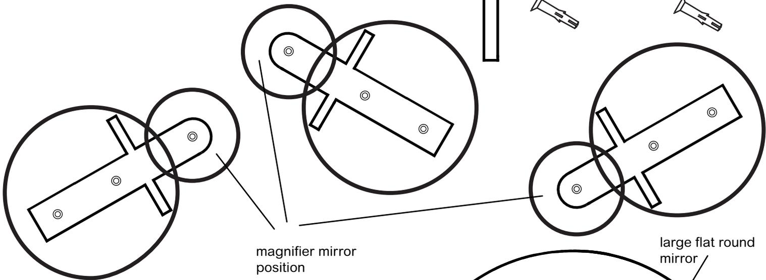
(B) Position the large flat round mirror over the backboard so that the mirror screws can be fixed from the side edge to the backboard and mirror. Tighten screws with a screwdriver.
