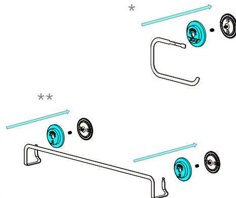
**7** Reassemble the bracket/s with the product attached (step 2). Make sure to tighten the caps firmly. **DO NOT OVER TIGHTEN.**
