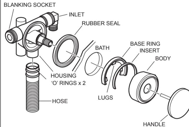
Prepare the assembly by pushing the 'O' ring onto the nut. Push the rubber seal onto the housing, and hold the unit in position from the outside of the bath. From the inside of the bath place the base ring over the bath hole, **if the hole is too small, snap off one of the lugs with a pair of long nose pliers**. Slide the insert and body into the base ring and screw on the nut, finally screw on the cover.
